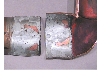
Figure 4: Trapped flux pockets: shiny, wet surfaces indicate the flux was trapped, not burned, an indication of improper technique
