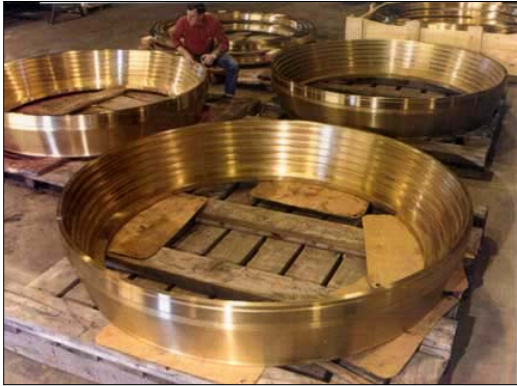
Photo 5. Wear rings for a large hydroturbine, centrifugally cast in nickel-aluminum bronze, alloy C95800. Nickel-aluminum bronze was selected for these rings, which operate under a hydrostatic head as large as 400 ft (122 m), for the alloy's proven anti-galling properties and excellent galvanic corrosion resistance with respect to the austenitic stainless steel (Type 304 and Nitonic 60) rotating runner components against which the rings operate. Passive nickel-aluminum bronzes are galvanically compatible with several corrosion-resistant ferrous materials, including titanium and its alloys. Rings of the type illustrated here have achieved more than 20 years of service in the Hoover, Grand Coulee, and other dams, and
