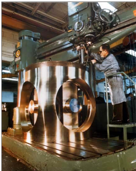
Photo 4. Nickel-aluminum bronze (alloy C95800) hub for a variable pitch naval propeller. The alloy was selected for its high strength, non-magnetic properties, cavitation resistance and galvanic compatibility with the propeller blades. Nickel-aluminum bronze exhibits good anti-galling characteristics against itself, an important property in this application since the propeller blades, which are also cast in nickel-aluminum bronze, rotate within the cylindrical openings on the sides of the hub. (Photo courtesy MetalTek, Inc., www.metalttekint.com )
