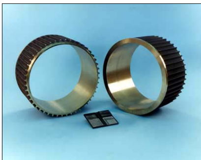
Photo 2. Clutch components for a shipboard winch, centrifugally cast in aluminum bronze alloy C95400. The inside diameter surfaces of these castings are actually metal-matrix composite structures containing non-metallic anti-wear particles, while the outer diameter is cast to net shape. Application of the continuous casting process to produce this innovative technique extended the life of the clutch component by 20-fold, and near net shape casting reduced the cost of finish machining. (Photo courtesy MetalTek, Inc., www.metaltelkint.com .)
