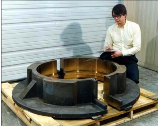
Photo 3. Propeller shaft seal, centrifugally cast in nickel-aluminum bronze. Alloy C95800 was specified for this application for its seawater corrosion resistance, non-magnetic properties and good anti-galling characteristics against steel (the propeller shaft). Small flats were intentionally cast into the blank, which was then cut transversely and finish machined to the proper inside diameter. Note that the outside diameter is cast to net shape and does not require further machining. (Photo courtesy MetalTek, Inc., www.metalttekint.com .)
