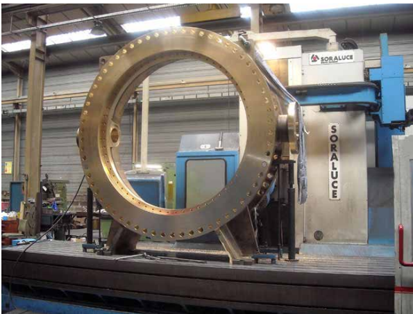
Figure 32 – Valve body 2000 mm dia 6000 kg (Courtesy Inoxyda SA, France)
