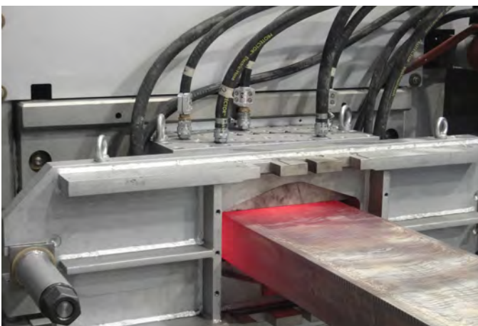
Figure 69 - Horizontal slab casting (Courtesy Alfred Wertli, Switzerland)
