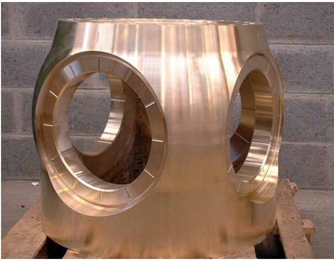
Figure 14 - Hub body 8500 kg (Courtesy Inoxyda SA, France)
