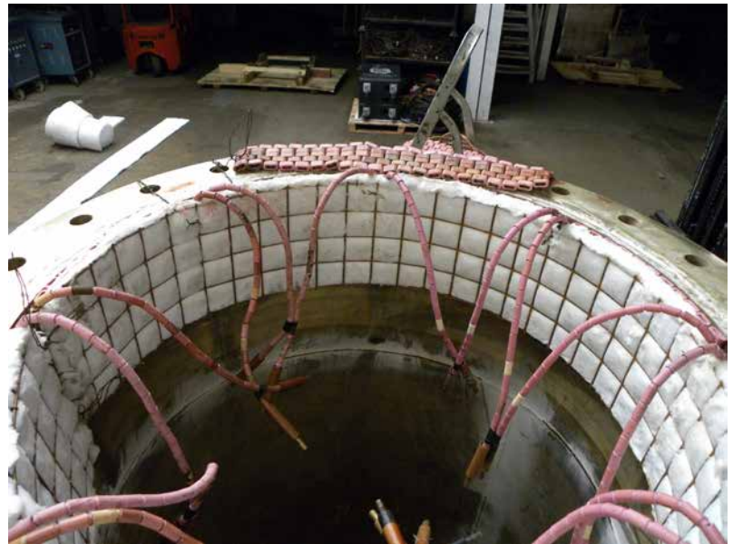
Figures 57 and 58 - Selective annealing heat treatment of a welded flange on a desalination pump housing using resistance heating elements, 675°C for six hours (Courtesy Site Heat Treatment, Port Talbot, and Copper Alloys Ltd, Stoke-on-Trent, UK)
