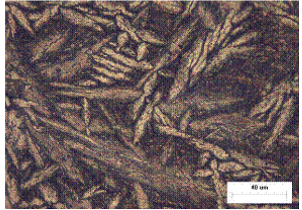
Figure 36 - CuAl10Ni5Fe4Mn DIN 2.0966 Widmanstätten martensitic structure. Water quenched from 900°C. Etched in acidified ferric chloride solution.
