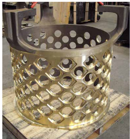
Figure 10 - Submarine acoustic antenna (Courtesy Inoxyda SA, France)
