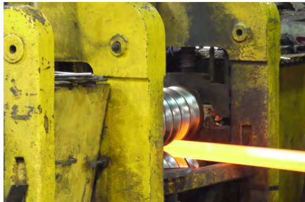
Figure 75 – Hot rolling (Courtesy Pro-Roll Ltd, Sheffield, UK)
