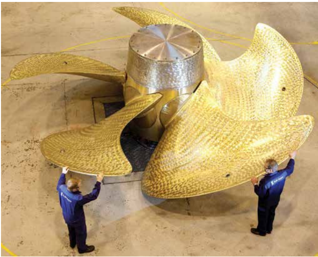
Figure 11 – Adjustable bolted propeller - one of two 33 tonne propellers from the Queen Elizabeth class aircraft carrier capable of producing 40 MW of thrust (Courtesy Rolls Royce Marine)
