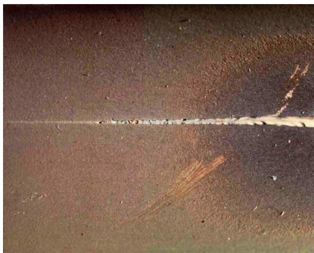
Figure 8 - Erosion corrosion of a scratch on an aluminium brass condenser tube due to excessive chlorination
