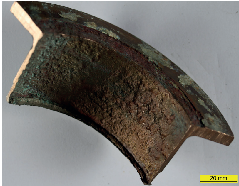
Figure 3 - Erosion corrosion of 90/10 copper-nickel after the weld on a weld neck flange due to excessive flow velocity (Courtesy of KME)
