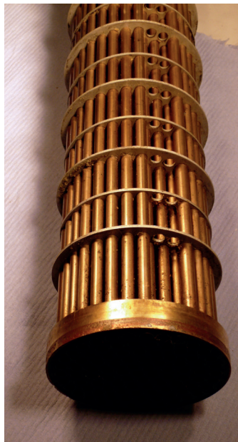
Figure 2 - 90/10 copper-nickel tubing in an oil cooler
